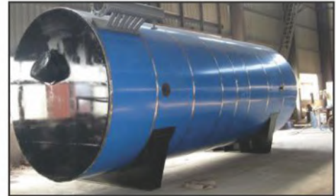
Thermal oil furnace
