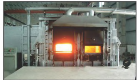
Aluminum melting furnace
